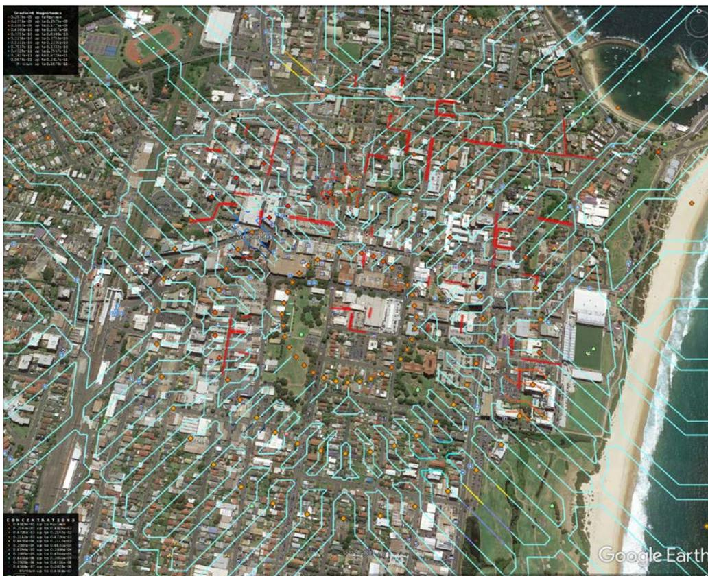
**Figure 4.** Plots of CO concentration across study area, generated by traffic on 100 road links (in red). Lines show gradients (legend at top), points are spot concentrations (lower legend).
